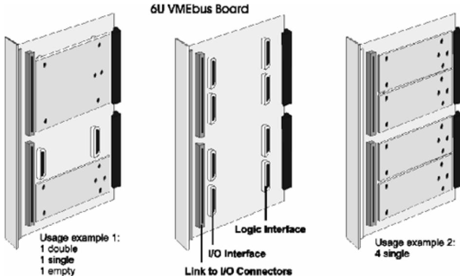
IndustryPack modules are available in *single* and *double* size. In its double size, the format is slightly larger than a PC•MIP module. A single IP measures 45.7 mm x 99 mm, (~1.8 x 3.9 inches), and a double IP measures 91.4 mm x 99 mm, (~3.6 x 3.9 inches). Components mounted on an IP module are allowed to have a maximum height of
