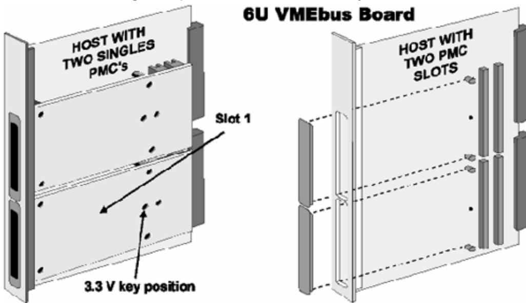
Mezzanine Card specification and fit a form factor of 74 mm x 149 mm, (~3 x 5 inches). A 3U VME Host can accept one PMC module, and a 6U Host will accept two modules side by side. Each PMC module uses two 64-pin PCI connectors as the Host interconnect and may use either one or two
